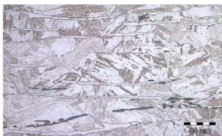
Homogenous microstructure of SIMOLD 2099 across the whole section of plate
