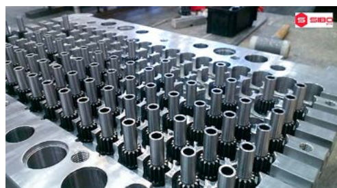
Mould base made of SIMOLD 2099 for plastic closures mould tool
