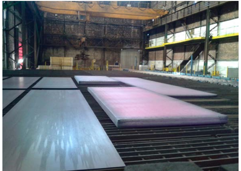
SIMOLD 2099 hot rolled plates cooled after rolling on Quarto plate mill
